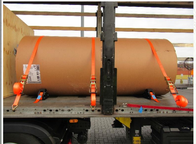
Image 9: Side view of two secured parallel positioned reels with a total weight \leq 10.000 kg.
